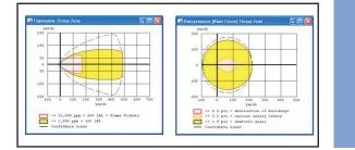
ALG staff have used accidental release dispersion models such as ALOHA to assess short-term impacts of releases from ruptured vessels and pipes for a variety of hazardous chemicals, including hydrogen sulfide, chlorine, anhydrous ammonia, and ethylene oxide. Additionally, for flammable gases and liquids, EPA/CEPPO-approved Offsite Consequence Analysis methods have been used to determine the effects of vapor cloud fires and explosions, pool fires, and BLEVEs.
