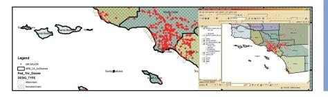
ALG uses the ArcGIS software for processing geographic information to use in HRAs. ArcGIS is used to identify locations of sensitive receptors (e.g., schools and hospitals), delineate areas of differing exposures (i.e., residential and workplace), and prepare base maps for presentation of results.
